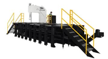
Actual Power Model: 0510-VS is a highly capable cutting tool designed for vertical cutting applications. This heavy-duty traversing head vertical plate saw is available to efficiently cut large solid plates and blocks with excellent accuracy. The machine is suitable for mass production.
